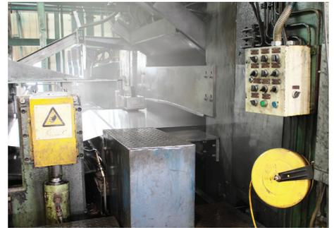
**Millmate Thickness Gauging (MTG) in the cold rolling mills**
