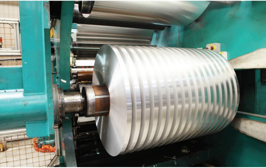
Gränges Shanghai's (former Sapa Shanghai) rolling mills and process lines are running with 6 Stressometer systems, 7 MTG-gauges, 2 Strip Scanner systems and around 30 tension load cells.
